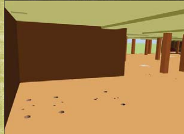
Translating X, Y, and Z coordinates from the BIM to northing, easting, and elevation points for the survey crew enabled direct, paperless use of 3D BIM data in the field to layout sleeves and embeds in the concrete.
