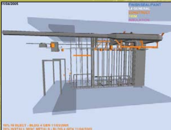
BIM was integrated with a detailed project schedule to communicate sequence of work to subcontractors.
