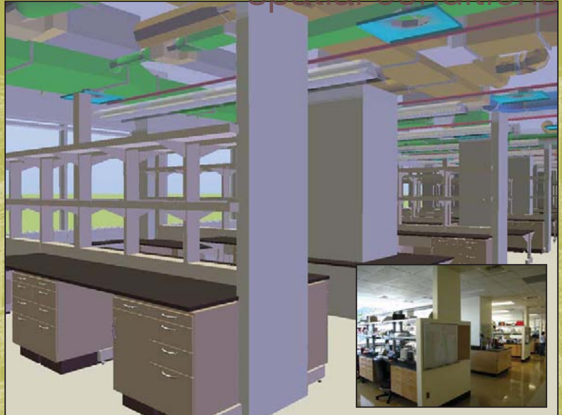
Real-time design visualization of the model provides end-users with an understanding of their proposed tenant improvements, and enables them to revise the design before it is built.
